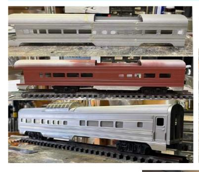
Dan Gory is closing in on the finished project: an extra-long dome cafeteria car, including custom 3D frames and roller bearings. wow.
